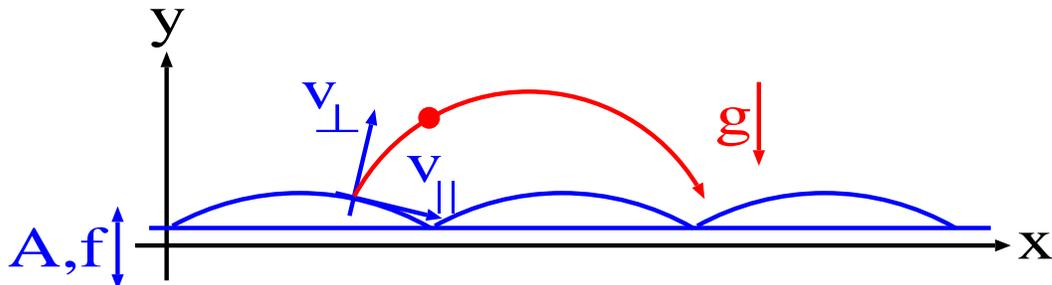
Fig. 1. Sketch of the bouncing ball billiard: A point particle collides inelastically with circular scatterers forming a periodic lattice on a line. Parallel to  $y$  there is an external field with constant acceleration  $g$ . The corrugated floor oscillates with amplitude  $A$  and frequency  $f$ .
