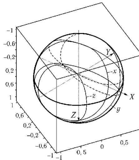
Fig. 27. Motion of the apices of the principal axes of a rigid body in the absolute space in Goryachev – Chaplygin case for the unstable periodic solution on branch II in Fig. 17, for a single value of an energy. Letters  $x, y, z$  denote the trajectories of the corresponding axes. (Motion for other values of energy do not differ qualitatively, therefore we do not present them.)
