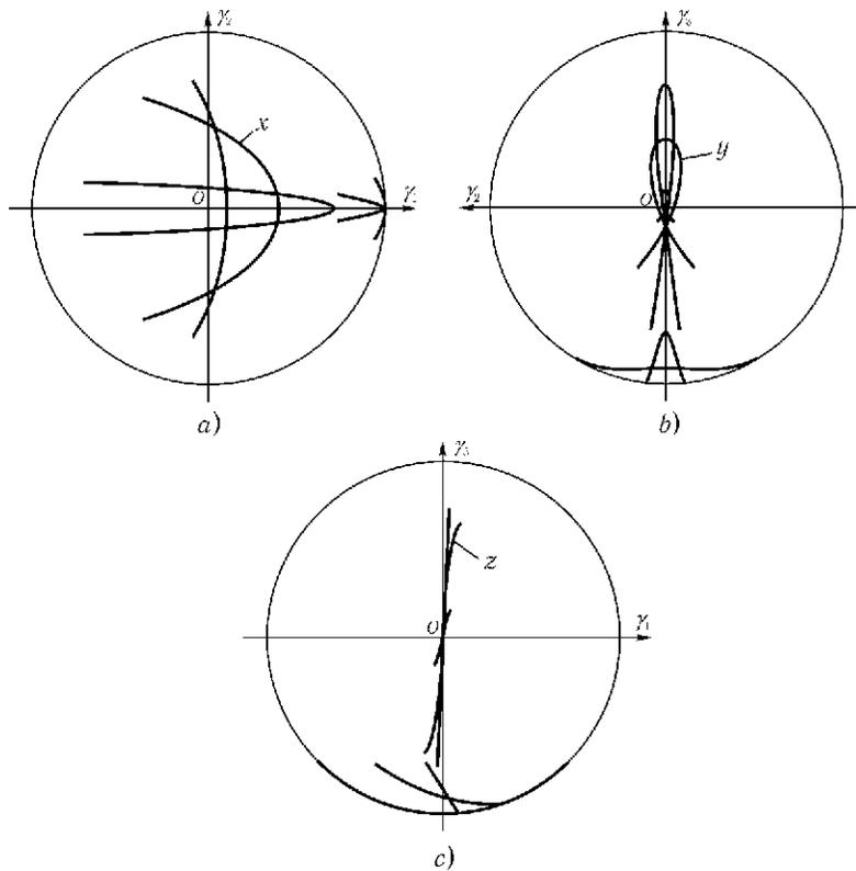
Fig. 22. This figure illustrates the behavior of the principal axes of a rigid body in the fixed frame of reference for Goryachev solutions at a fixed value of energy  $h < 1$  ( $h = -0.7$ ). It can be clearly seen that this solutions are *periodic* in the absolute space, which with the increase of parameter  $b$  changes from oscillations in plane  $Oxy$  to oscillations in plane  $Oxz$ . (Letters  $x, y, z$  denote the axes bound with the body.)
