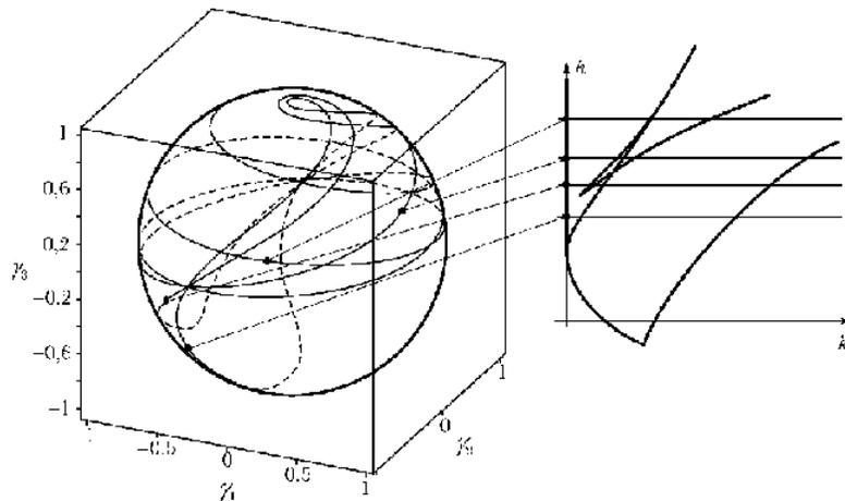
Fig. 6. Delone Solution. Motion of the unit vector  $\gamma$  for the nonzero value of area integral ( $c = 1.15$ ) and for various values of energy  $h$ .
