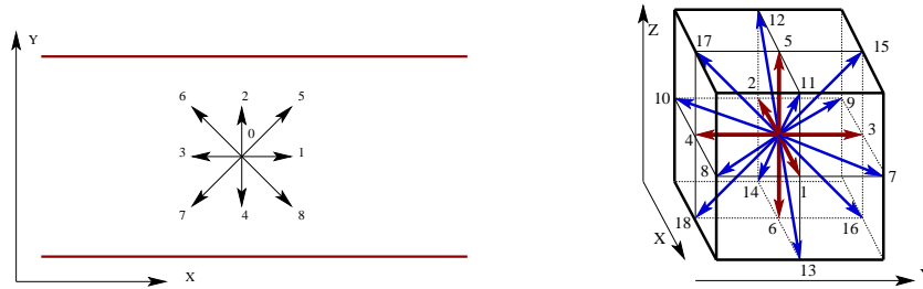
Figure 10: 2d and 3d lattice discretization of the velocities in the LBE schemes used in this work. The velocities entering in the north wall in the 2d scheme (left) are, f_5, f_2, f_6 . The outgoing velocities are: f_7, f_4, f_8 . At the south wall the roles are exchanged.
