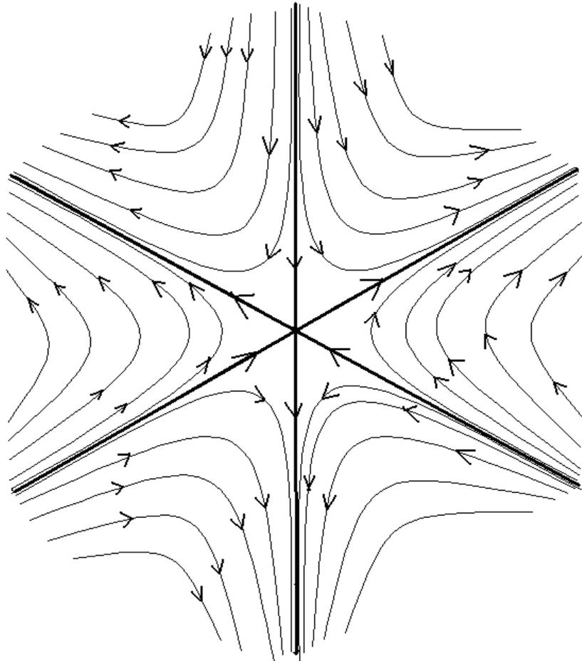
*Fig. 2.3 Vector field near singular point with  $m=3$*
