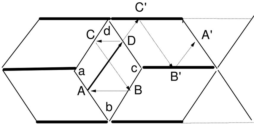
***Fig.3.4: The periodic orbit (ADCBA) in the rhombus  $abcd$  is equivalent to the periodic orbit (ADC'B'A') in the barrier billiard, which closes on equivalent point on the other plane.***
