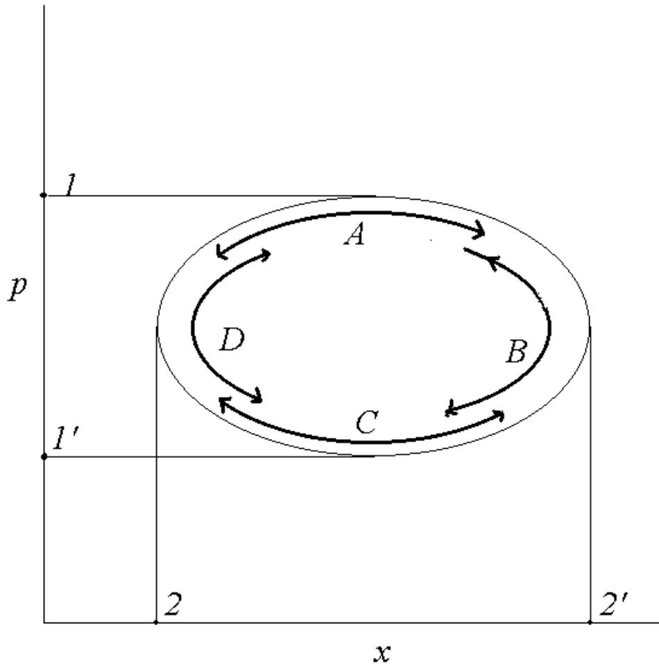
*Fig. 1.3: In one degree of freedom, configuration space caustics (2&2') and momentum space caustics (1&1') never occur at the same place. In higher degrees of freedom also there always exist a representation in which a given point is caustic free. Thus a Lagrangian manifold can always be covered by overlapping regions (e.g. A,B,C,D) that are caustic-free.*
