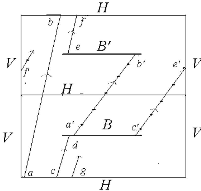
Fig. 3.11: H-M billiard (pqrs). Fundamental region requires two replicas as shown. V,H represents identified sides of a periodic cells. B,B' are barriers in respective cells. A trajectory abcdefg... starts at 'a', meet H at 'b', due to identification it is then transferred to 'c' and so on. Note that 'd' is equivalent to 'e' since lower side of B is identified with upper side of B' and vice versa.
