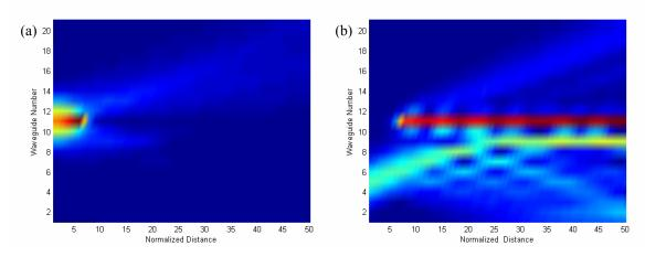
Fig. 3. Simulation of energy transfer and beam steering. The blocking beam in a) disappears, generating the SRS beam shown in b), and the subsequent beam steering of the input signal.
