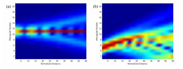
Fig. 2. Simulation of the independent propagation of the (a) input blocker beam at waveguide array center and (b) Raman signal beam applied several waveguides below the center, with an input tilt. The signal beam illustrates the expected nonlinear discrete diffraction.
