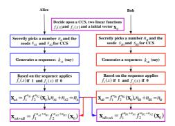
Fig.1. (color online). The proposed key exchange protocol using CCS.
