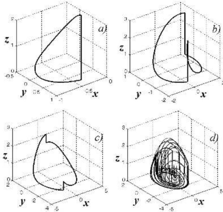
Figure 6: The portraits of nonautonomous attractors of Rössler system (2). Attractors are plotted for the next pulsed amplitude and period: a)  $A = 5$  and  $T = 2.85$ ; b)  $A = 2.4$  and  $T = 2.85$ ; c)  $A = 0.5$  and  $T = 2.85$ ; d)  $A = 1$  and  $T = 4.5$ .
