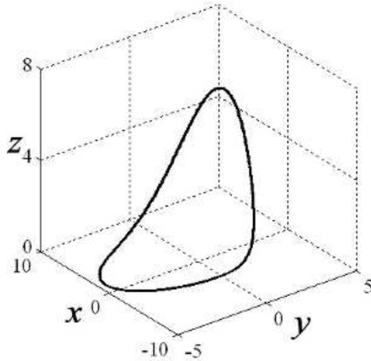
Figure 1: Attractor for the autonomous Rössler system. Attractor is plotted for  $p = 0.2$ ,  $q = 0.1$  and  $r = 1.5$ .
