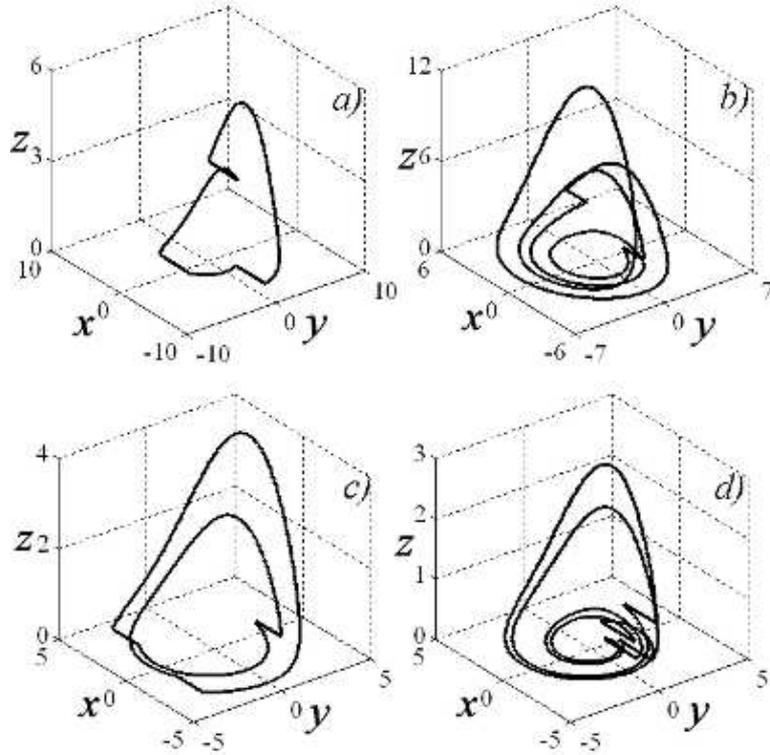
Figure 3: The portraits of nonautonomous attractors of Rössler system (1). Attractors are plotted for the next pulsed amplitude and period: a)  $A = 4.4$  and  $T = 1.8$ ; b)  $A = 1.8$  and  $T = 10.9$ ; c)  $A = 2$  and  $T = 3.7$ ; d)  $A = 2.5$  and  $T = 7.1$ .
