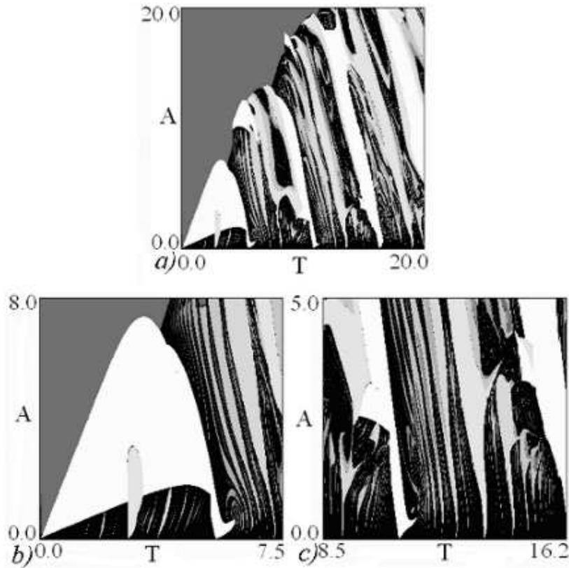
Figure 5: The chart of dynamical regimes and its fragments on the  $A - T$  parameters plane, constructed for nonautonomous Rössler system (2) with the parameters  $p = 0.2$ ,  $q = 0.1$  and  $r = 1.5$ .
