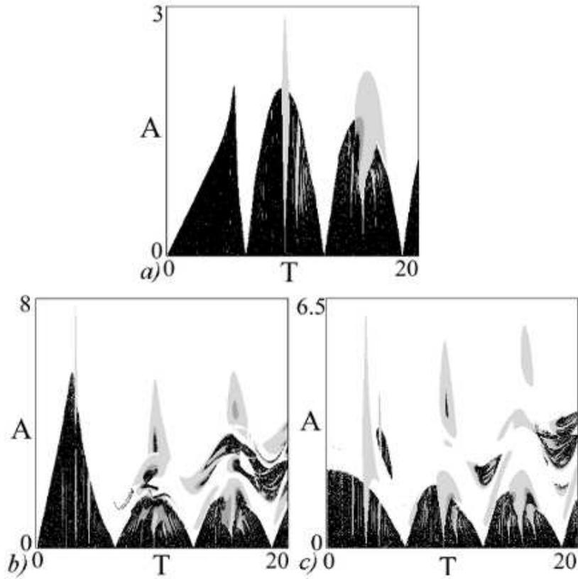
Figure 9: Charts of dynamical regimes of the nonautonomous Dmitriev - Kislov generator on the  $A - T$  plane. Charts are plotted for the cases, when pulses act along the  $x$  axis (fig.a), the  $y$  axis (fig.b) and the  $z$  axis (fig.c). Systems parameters are fixed at  $D = 6$ ,  $M = 5.5$  and  $Q = 10$ .
