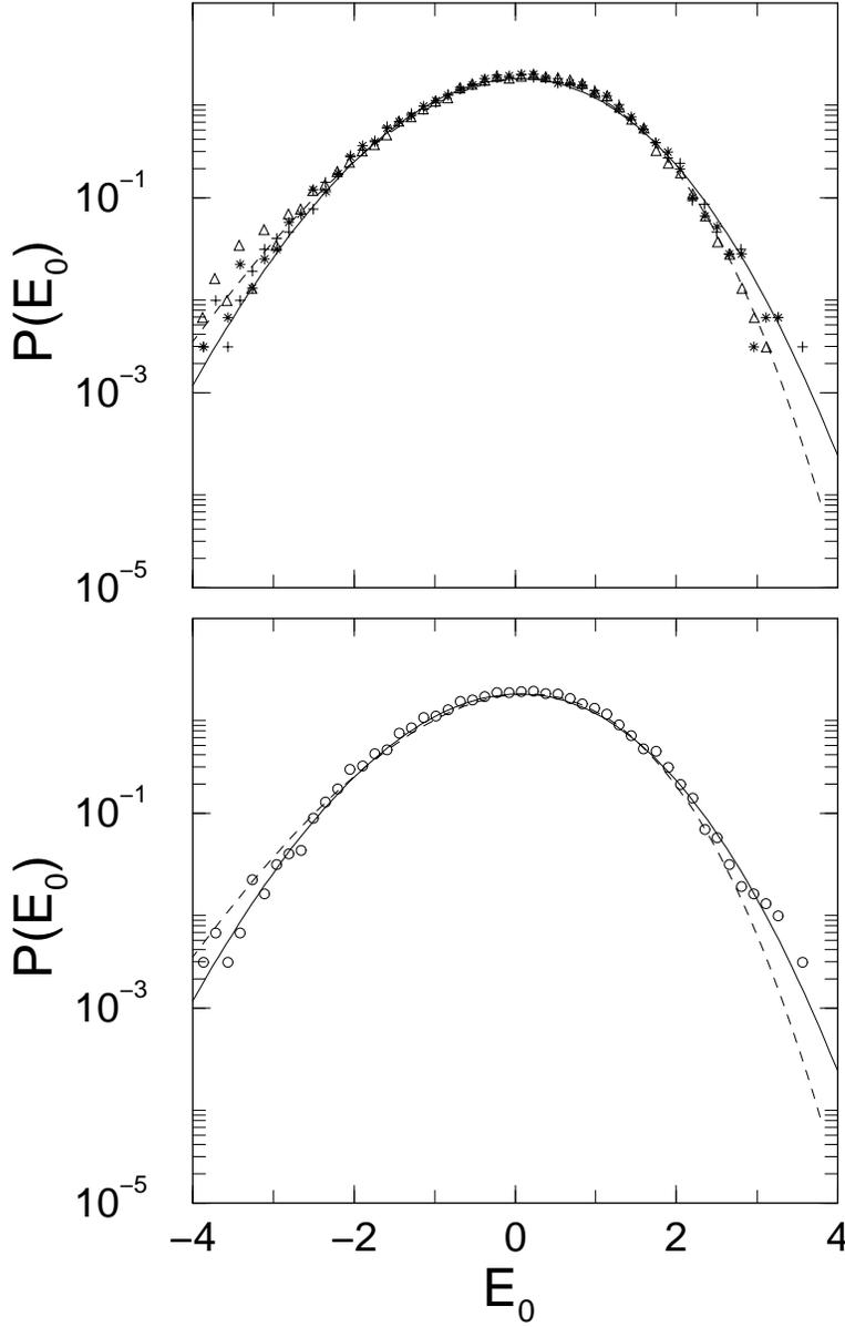
FIG. 4. Top panel: Distribution of the ground state energy for the IEM for  $N_p = 4$  (triangles), 5 (crosses) and 6 (stars). Bottom panel: Distribution of the ground state energy for the IEM at half filling,  $N_p = 7$  (circles). In both panels, solid and dashed lines give the distribution for the  $N = 2$  and  $N = \infty$  GOE respectively. The particle statistics plays a role at half-filling only, rendering the distribution closer to the  $N = 2$  GOE.
