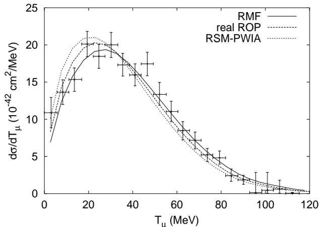
FIG. 5: Observed distribution of muon kinetic energies  $T_\mu$  compared with the flux-averaged predictions of our RSM, in PWIA (dotted line) and including FSI within the RMF (solid) and purely real ROP (dashed) frameworks. The theoretical distributions have been normalized to give the same integrated values as the experimental points, and have been folded in energy with a bin size of 5 MeV, the same employed for the experimental data. Data are from Albert et al. [12].
