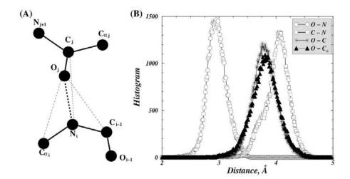
**Figure 6:** (A) The schematic diagram of the hydrogen bond among backbone. Only the backbone beads of the model are shown. The thick dash lines represent the hydrogen bonds and the thin dashed lines indicate the auxiliary constraints for the formation of hydrogen bond. (B) The histogram of distances between the hydrogen bonded oxygen and nitrogen as well as the distance of the auxiliary constraints, which is calculated for the hydrogen bonds in crystal structures.
