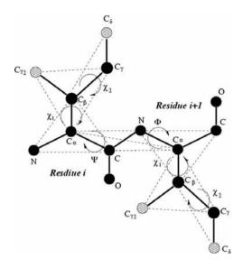
**Figure 1:** The schematic diagram of the model peptide. Only two consecutive residues are presented. The shaded second gamma and delta beads  $-C_{\gamma 2}$  and  $C_{\delta}$  – indicate that not all amino acids have them. Covalent bonds are represented as thick lines and the constraints that need to fix the bonds angles and the planar property of peptide bonds are denoted as thin dashed lines.
