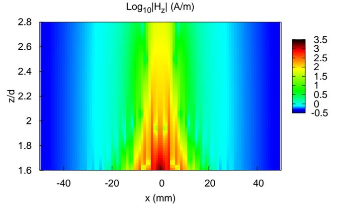
FIG. 2: Map of  $\log_{10} |H_z|$  corresponding to the field generated at the back side of the lens by a source loop antenna shown in Fig. 1. The slab is made of a left-handed medium of thickness  $d = 4$  mm with  $\epsilon = \epsilon_0 = \epsilon_0 = -1 + i0.001$ , and is separated a distance  $z = d/2$  from the source. The source is considered, for simplicity, a *circular* loop antenna of radius  $r_1 = 5$  mm. The wire radius is of  $0.2$  mm. The operation frequency is 3 GHz.
