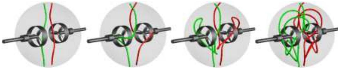
FIG. 4: (color) The mechanism of field generation in a laminar double-vortex flow is modeled in the frozen flux limit ( $Rm \rightarrow \infty$ ). A field line directed through the equator is stretched by the poloidal flow towards the pole and then twisted back onto itself by the toroidal flow.
