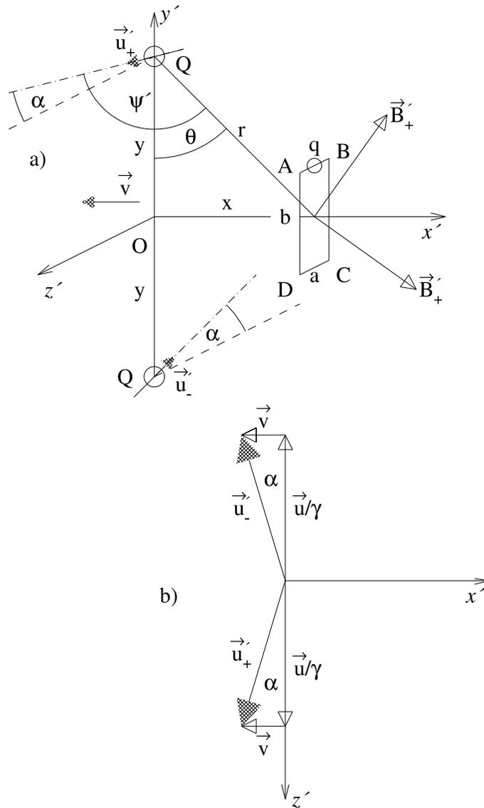
Figure 2: Geometry for calculation of electromagnetic induction in the frame  $S'$  in which the test charge is at rest and the magnet moves at velocity  $\vec{v}$  parallel to the  $-x$ -axis. Distances, angles, velocity vectors and magnetic fields are defined in a manner similar to those in Fig.1. a) shows a perspective view and b) the  $x'$ - $z'$  projection.
