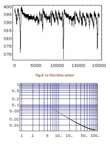
Fig.8.1b The power spectrum of the time series presented in Fig.8.1a
