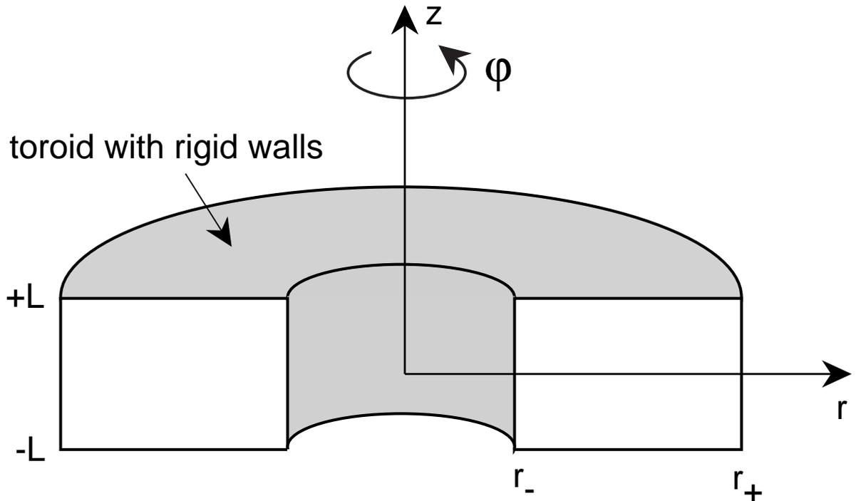
FIG 1. Geometry of computational model. The toroid has a rectangular cross section with impenetrable, perfectly conducting, perfectly smooth walls. The magnetofluid occupies the region between the radii  $r_-$  and  $r_+$ , and the planes  $z = \pm L$ .
