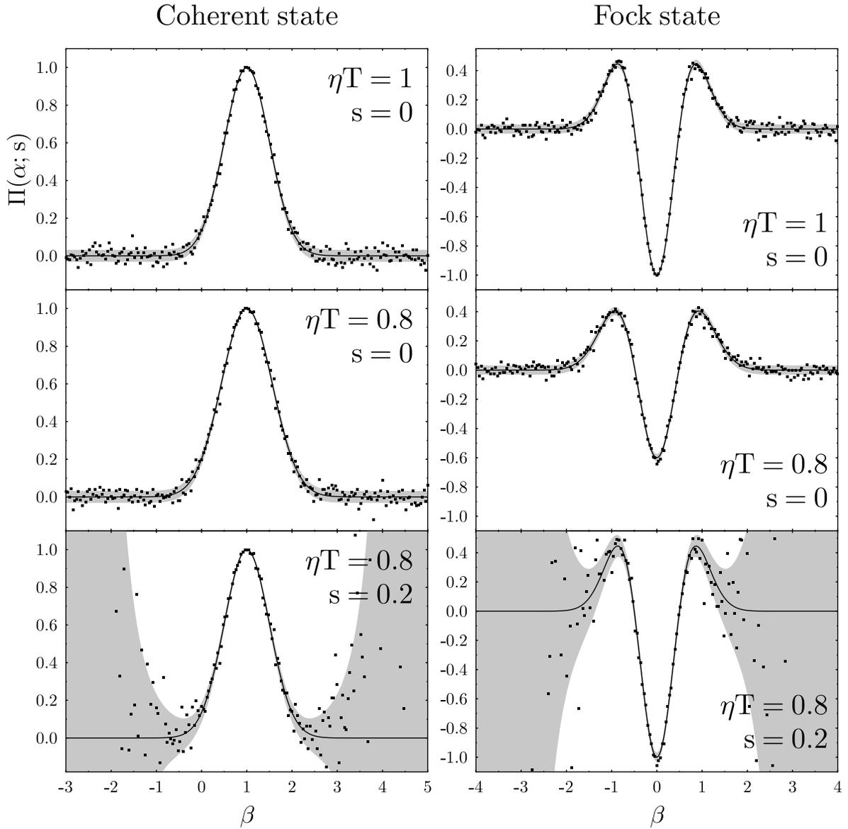
FIG. 4. Reconstruction of the quasiprobability distributions of the coherent state  $|\alpha_0 = 1\rangle$  (left) and the one photon Fock state (right) from  $N = 1000$  events. The solid lines are the analytical quasidistributions and the grey areas mark the statistical dispersion.
