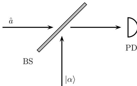
FIG. 2. The experimental setup proposed to measure quasidistribution functions. The signal  $\hat{a}$  is superposed by the beam splitter BS on a coherent state  $|\alpha\rangle$ . The photon statistics of this superposition is measured by the photodetector PD.
