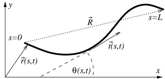
FIG. 1: Sketch of a polymer of length  $L$ , represented by a continuous space curve  $\mathbf{r}(s;t)$ . An example is shown for the local unit tangent vector  $\hat{t}(s;t)$ , as well as the end-to-end distance vector  $\mathbf{R}$ .
