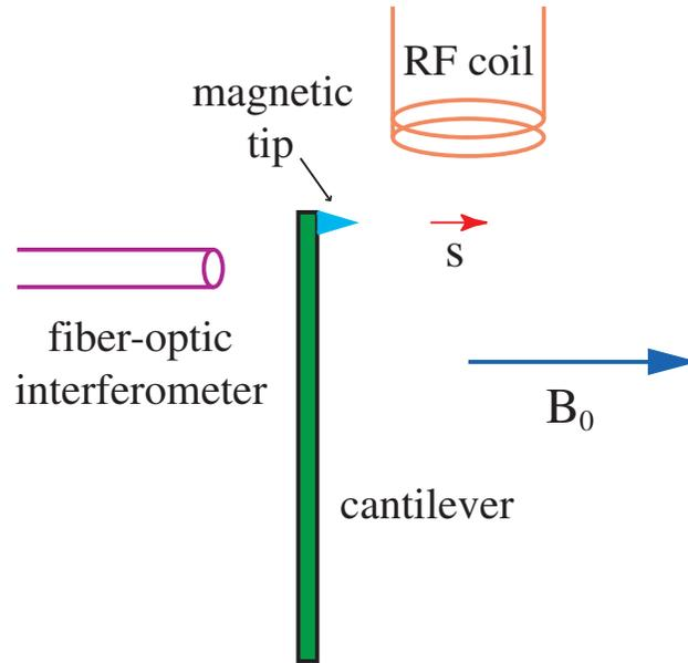
Figure 1: Schematic diagram of the MRFM setup.
