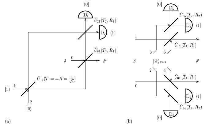
FIG. 3: Setups consisting of beam splitters  $\hat{U}$  and photodetectors  $D$ , conditionally implementing a desired binomial in  $\hat{n}_0$  (a) and a desired binomial in  $(\hat{n}_1 \hat{n}_0)$  with some given (b).
