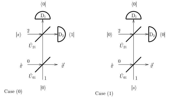
FIG. 1: Setup consisting of beam splitters  $\hat{U}$  and photodetectors  $D$  and implementing conditional subtraction [case (0)] or addition [case (1)] of a photon on a signal state  $\mathcal{S}$ , each controlled by the photon number  $s = 0; 1$  of the Fock state  $|s\rangle$ , respectively. Note that in case (1) the beam splitter  $\hat{U}_{21}$  is redundant.
