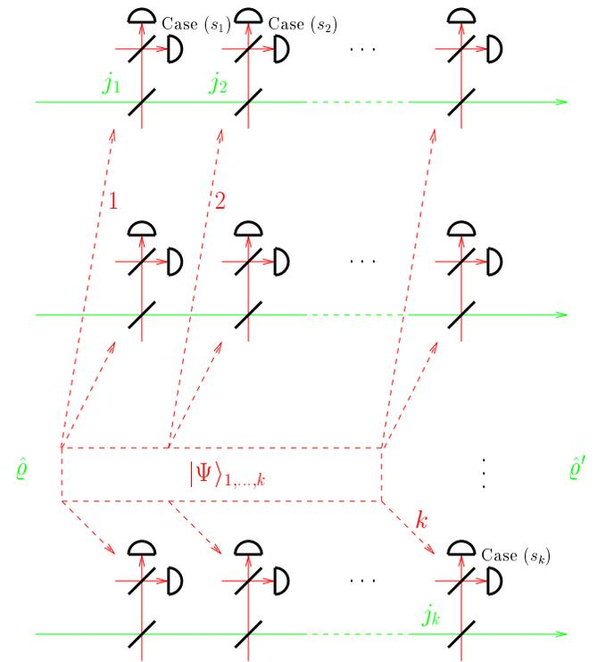
FIG. 2: Example of the overall setup consisting of  $k$  devices Fig. 1 applied in the signal modes  $j_1, \dots, j_k$  in cases  $(s_1), \dots, (s_k)$ , respectively. These modes do not have to be distinct from another. The respective control input ports of the devices which are fed with states  $|j_i\rangle$  in Fig. 1, here share an entangled state  $|j_{i_1, \dots, i_k}\rangle$  given by Eq. (6).
