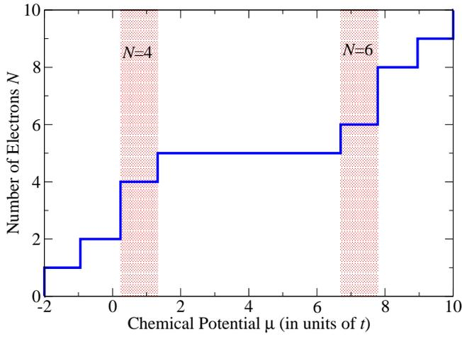
FIG. 2: Total occupancy  $N = \sum_i n_i$  of the 5-dot system as a function of overall chemical potential  $\mu$ . Here  $t_{ij} = 1$ ,  $U_i = 8$ , and  $\epsilon_i = 0$ . The ground state is a doubly degenerate singlet when the system is filled with 4 or 6 electrons.
