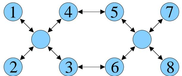
FIG. 5: A two-qubit operation can be performed by tuning on tunneling between two pairs of dots in neighboring composite qubits. Combined with the single-qubit rotations in Fig. 4, this operation allows any arbitrary unitary transformation to be performed.
