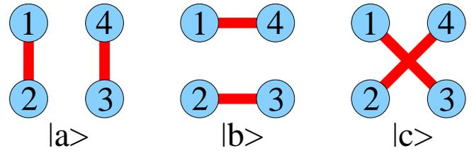
FIG. 3:  $G$  ground states of the 5-dot composite qubit. In each eigenstate, the middle dot is omitted. The lines connecting dots represent singlet valence bonds when both dots are occupied. These three states are not orthogonal: two orthogonal states may be formed, for example, as  $|\bar{j}_i = \bar{j}_i\rangle$  and  $|\bar{j}_i = (\bar{j}_i + \bar{j}_i)\rangle = \bar{3}$ .
