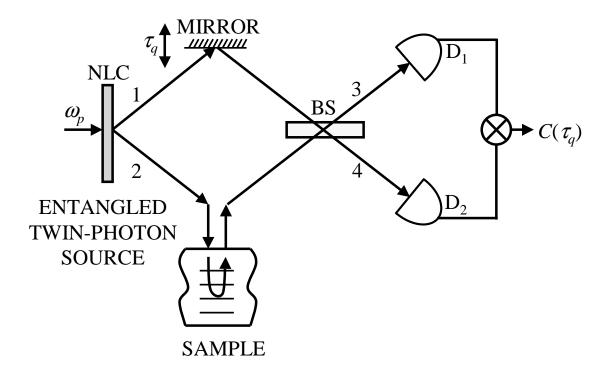
FIG.1: Schem atic of quantum -optical coherence tom ography (QOCT). A monochrom atic laser of angular frequency  $!_p$  pumps a nonlinear crystal (NLC), generating pairs of entangled photons. BS stands for beam splitter and  $_q$  is an adjustable temporal delay. D<sub>1</sub> and D<sub>2</sub> are single-photon-counting detectors that feed a coincidence circuit indicated by the symbol<sup>N</sup>. The outcome of an experiment is the coincidence rate C ( $_q$ ).
