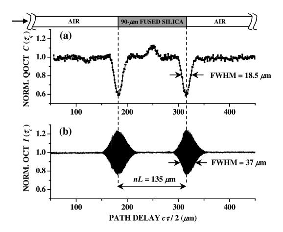
FIG. 3: QOCT and OCT normalized interferograms for a 90-m fused-silica window in air (as shown at top of gure). The abscissa is the scaled temporal delay c = 2, which represents displacement of the delay line (therefore represents both  $_{\rm q}$  and  $_{\rm c}$ ). (a) Coincidence rate C ( $_{\rm q}$ ) normalized to  $_0$  (the QOCT normalized interferogram). (b) Singles rate I ( $_{\rm c}$ ) normalized to constant background (the normalized OCT interferogram).
