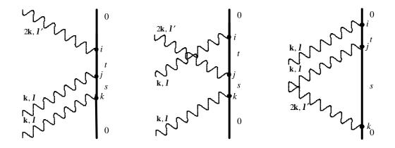
Figure 1: The three time ordered diagrams for second harmonic generation
