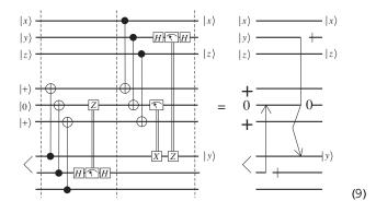
The initial Bell state preparation is done by a single recovery as in (3), so the complete network requires 3 time steps, these are shown separated by dashed vertical lines.
