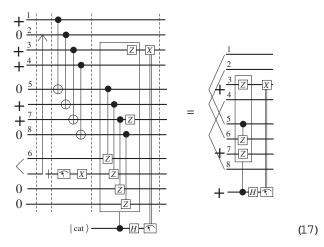
where the diagram on the right explains the logical e ect of the fault-tolerant diagram on the left. Bit number 6 has been left in a separate block so that if the  $^{\rm CZ}$   $^{56}$  gate in (16) is needed then it can be implemented immediately. To m inim ise the number of online time steps bit 7 should also be positioned in a separate block. This can be done
