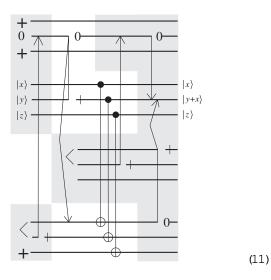
The shaded area is the o ine part, where, as discussed in section IIA, we count the initial teleportation (from m em ory' to 'accum ulator') as online, and the nal teleportation (from 'accum ulator' to mem ory') as o ine.
