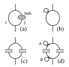
FIG. 1: Various setups of two-slit interferom etry (a) with the path 2 containing a usual external bath denoted by the grey circular region, (b) with no bath but delay, (c) with two paths containing the sam e nonlinear regions denoted by the grey boxes. (d) The sam e as (c) with delay in one of the paths after (A) and before (B) the interaction within the nonlinear region.
