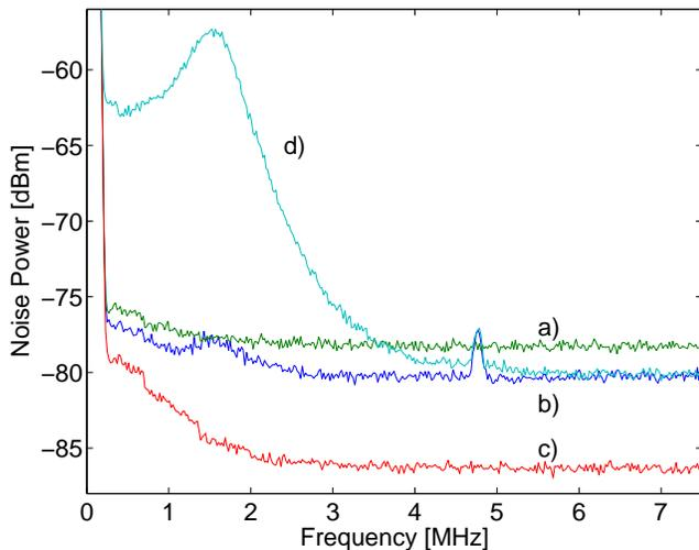
FIG. 2: Measured noise power spectra at sideband frequencies  $\Omega/2\pi$ . The distances between the shot-noise curve (a) and curves (b) and (d), respectively, represent the directly observed squeezing. The distance between curves (b) and (d) represents the optical cancellation of technical noise achieved. (c) represents the detector dark noise.
