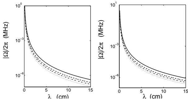
FIG. 1: Rabi frequency  $|\Omega|$  versus the microwave wavelength  $\lambda$  for a full-wavelength cavity (a) and a quarter-wavelength cavity (b) with ratios  $E_{\text{ch}}/E_J = 4$  (top solid line), 7 (dashed line), 10 (dashed-dotted line), 15 (bottom dotted line), respectively.
