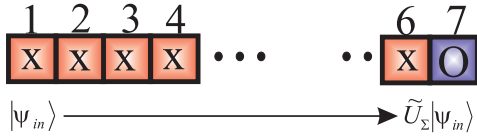
FIG. 7: Information flow through an N -qubit linear cluster.
