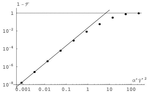
FIG. 3: The infidelity,  $1 - \mathcal{F}$  versus non-dimensional diffusion parameter  $\alpha^* \bar{\gamma}^{*2}$ . Points are from numerical calculation using a cavity to simulate a dispersive medium. Solid line is the analytic result, taken from [4]. When the dispersion becomes dominant, the infidelity (i.e. error) asymptotes to unity.
