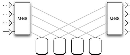
FIG. 2: Fermionic dispersion treated using  $M$ -port beam splitters to direct modes onto separate cavities, which are subsequently recombined. Dotted lines represent unoccupied modes, and grey lines indicate weakly occupied modes.
