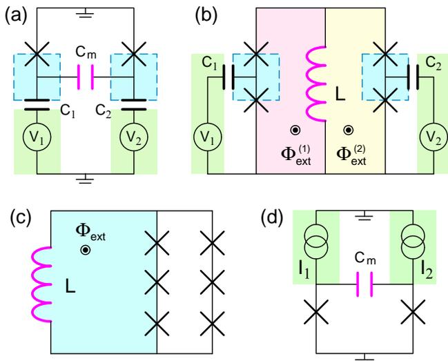
FIG. 4: **Coupling qubits.** (a) Two charge qubits (blue) coupled by a mutual capacitance  $C_m$  between the two boxes. (b) Two charge qubits coupled by a shared inductance  $L$ ; each box (blue) is connected to two Josephson junctions instead of one. (c) Two three-junction flux qubits coupled by the common inductance  $L$ . (d) Two phase qubits coupled by the mutual capacitance  $C_m$  between them.
