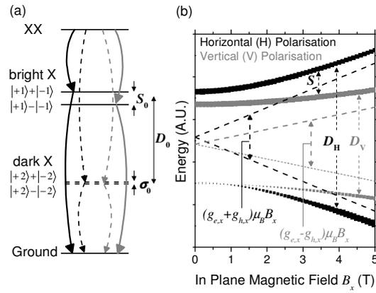
Fig. 1 (a) Energy level schematic of a single quantum dot. (b) Fine structure of the exciton state (X) in a single quantum dot as a function of in-plane magnetic field  $B_x$ . The size of the black (grey) points represents the fraction of horizontal (vertical) polarisation. The areas of the points corresponding to darker states has been multiplied by 5 for clarity.
