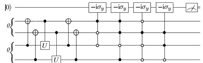
FIG. 3: Network estimating the second moment of partially transposed two-qubit density matrix  $\varrho$ .  $U_{\mathcal{H}'}$  is decomposed to single qubit gates; here  $U = (1/\sqrt{2})(\mathbb{1}_2 + i\sigma_y)$ .
