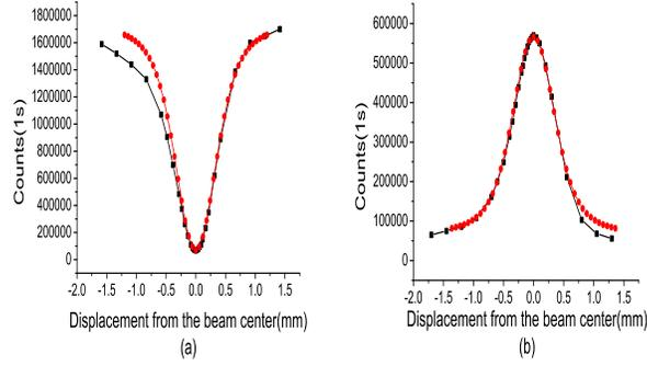
Fig. 3. Counts(square dots) as a function of the displacement of the second CGH. The metal plate is moved out. (a) The fork of first CGH is displaced far away from the beam center, so the light is in  $|0\rangle$  OAM state. (b) The fork of first CGH is placed in the beam center, so the light is in  $|1\rangle$  OAM state. The round dots come from theoretical calculation.
