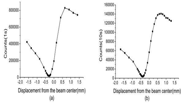
Fig. 5. Counts as a function of the displacement of the second CGH. The fork of first CGH is displaced a small amount from the beam center, so the light is in superposition mode. (a) The metal plate is moved out from the twin-lenses. The visibility is 96.0%. (b) The metal plate is placed between the twin-lenses. The visibility is 94.4%.
