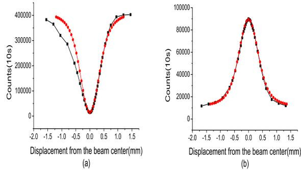
Fig. 4. Counts(square dots) as a function of the displacement of the second CGH. The metal plate is placed between the twin-lenses. (a) The fork of first CGH is displaced far away from the beam center, so the light incident on the metal plate is in  $|0\rangle$  OAM state. (b) The fork of first CGH is placed in the beam center, so the light incident on the metal plate is in  $|1\rangle$  OAM state. The round dots come from theoretical calculation.
