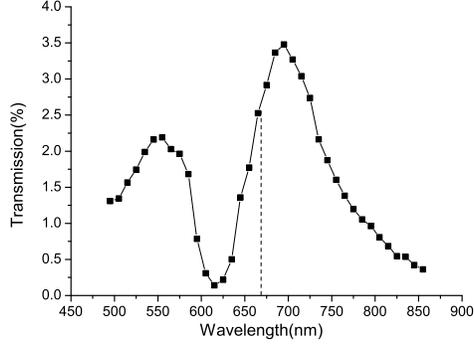
Fig. 1. Hole array transmittance as a function of wavelength. The dashed vertical line indicates the wavelength of 670nm used in the experiment.
