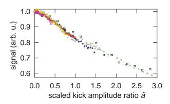
FIG. 2: (Color online) Number of zero-velocity atoms as a function of the scaled kick series amplitude ratio,  $\tilde{a} = aK^2/k^2$ . One observes the superposition of all curves. Parameters and graphic conventions are the same as in Fig. 1.
