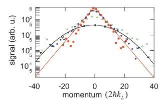
FIG. 3: (Color online) Experimentally observed momentum distributions at a = 0.25 in log scale, for various values of k and constant K = 6.8. The curve for k = 3.46 which corresponds to  $\tilde{a} = 0.97$  is well fitted by an exponential, whereas the curve with k = 1.44, or  $\tilde{a} = 5.6$  is fitted by a Gaussian.
