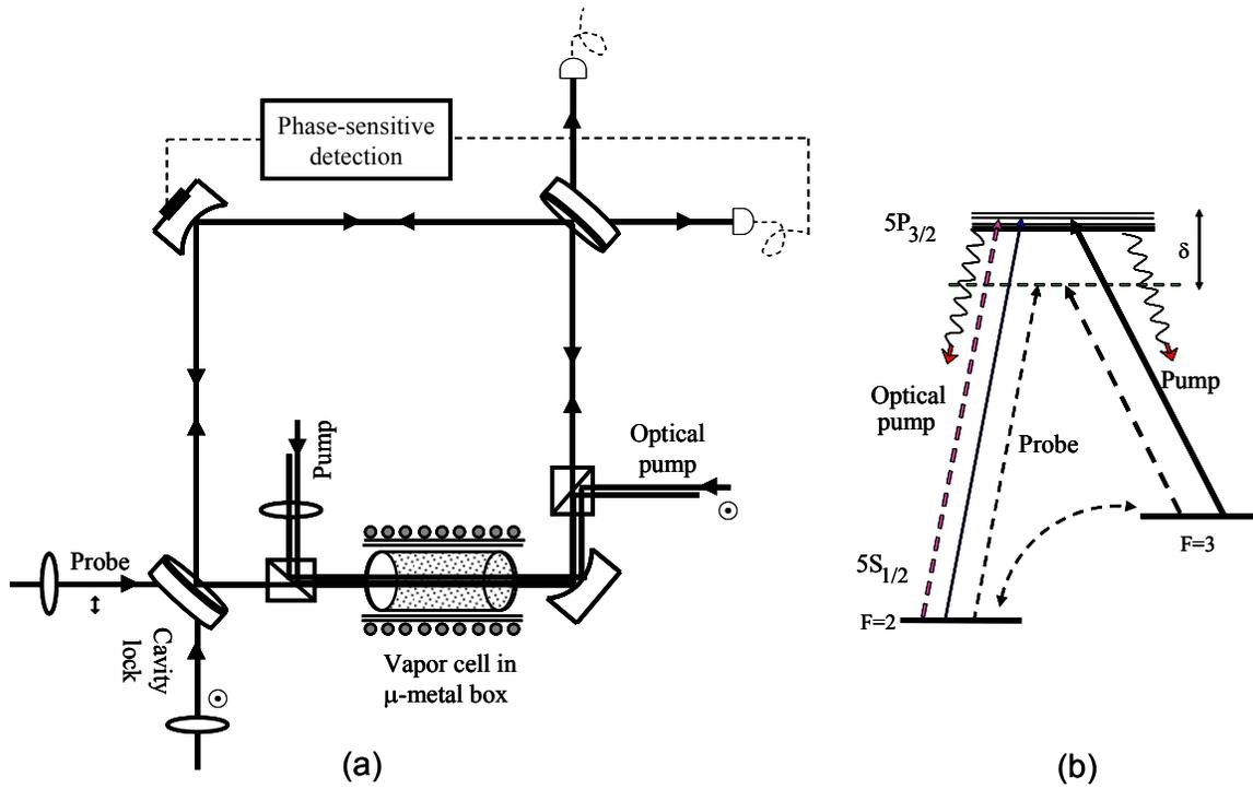
Fig.1 (a) Schematic of experimental set-up (b) two-photon transitions used in  $^{85}\text{Rb}$   $D_2$  line for EIT (solid lines) and Raman gain (dashed lines)
