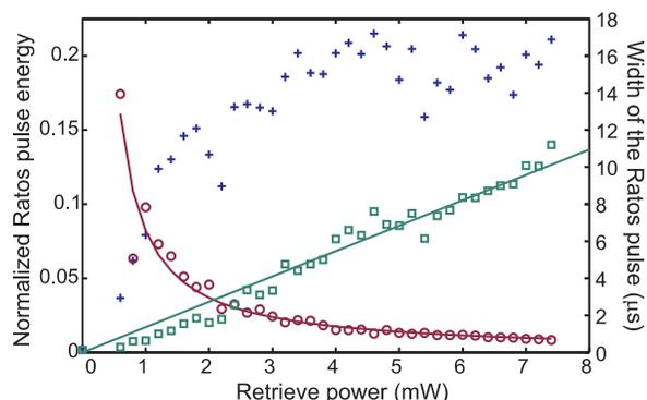
Fig. 3. Peak power of the retrieved Ratos pulse ( $\times$ ), its temporal width ( $\square$ ), and energy ( $\circ$ ) as a function of the power of the retrieve laser. The energy is normalized to the energy of the slowed down pulse. The peak intensity plot is in arbitrary units. The solid lines are a linear and inverse linear fits.
