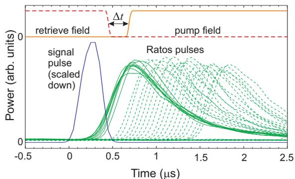
Fig. 2. Temporal profiles of the fields. Ratos pulses are shown for the case the retrieved field is turned on before (solid lines) and after (dashed lines) the pump field has been turned on.
