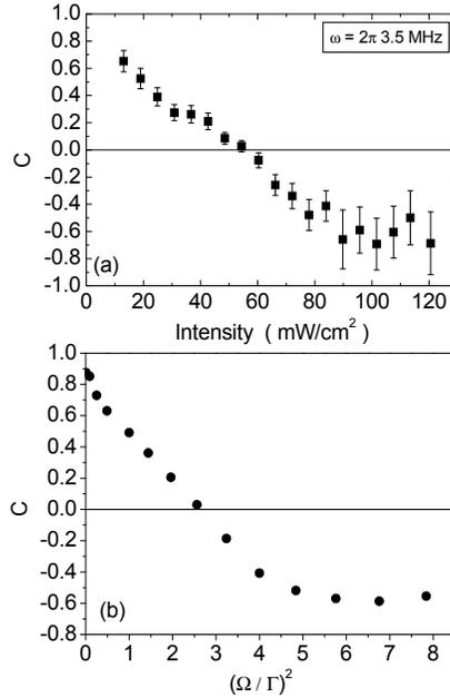
Fig. 3. Variation of the correlation coefficient with laser intensity (per beam) for an analysis frequency of 3.5 MHz. (a) Experiment. RBW = 1 MHz and VBW = 3 kHz. Each point is an average over  $6 \times 10^4$  measurements. (b) Theory (as described in x4.2).  $\gamma$  is the spontaneous emission decay rate from the excited state ( $\gamma = 2 \times 6 \text{ MHz}$ ). Other parameters are  $\omega_1 = \omega_2 = 2 \times 28.6 \text{ MHz}$ ,  $b_1 = b_2 = 0.08$ ,  $\epsilon = 0.02$ .
