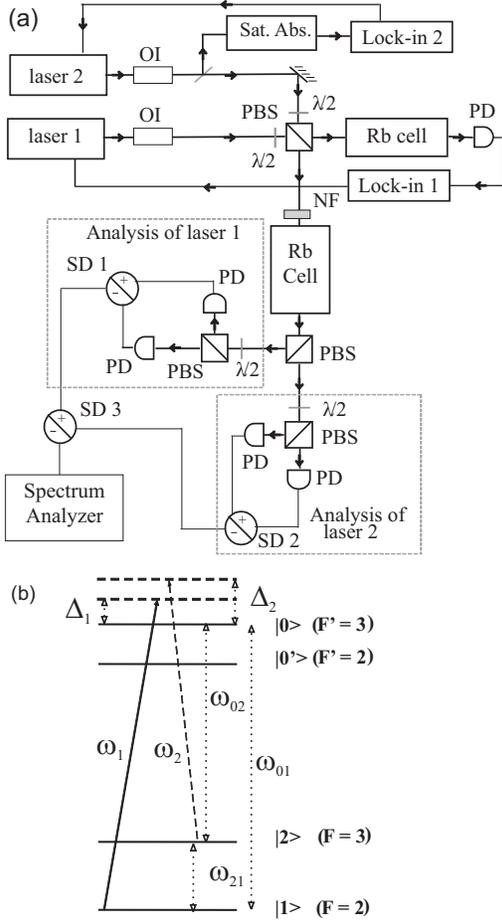
Fig. 1. (a) Experimental setup. The saturated absorption setup for laser 2 is not shown. OI: optical isolator; PBS: polarizing beam splitter; PD: photo-detector; NF: neutral filter;  $\lambda/2$ : halfwave plate. (b) Energy level representation for our atomic model and its correspondence to the relevant Rb hyperfine states. Solid line represents the pump field with frequency  $\omega_1$ ; dashed line represents the probe field with frequency  $\omega_2$ .
