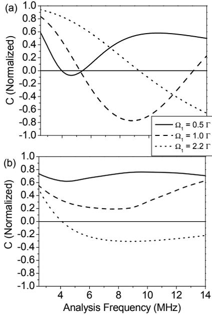
Fig. 6. Numerical results of the correlation coefficient as a function of the analysis frequency for various Rabi frequencies ( ) in the case of a 3-level atom at rest (a) and for a Doppler broadened ensemble (b).  $\Omega_1 = 0.5 \Gamma$  (solid),  $\Omega_1 = 1.0 \Gamma$  (dashed),  $\Omega_1 = 2.2 \Gamma$  (dotted).  $\Omega_2 = 1.12 \Omega_1$ ;  $\Omega_2 = 6 \text{ MHz}$  for  $^{85}\text{Rb}$ ,  $b_1 = b_2 = 0.08$ ;  $\delta = 0.02$ ,  $\gamma_1 = \gamma_2 = 0$ .
