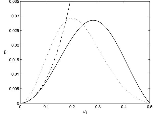
FIG. 9: Production rate  $r$  as a function of  $\epsilon$ . The dotted line corresponds to  $\eta_t = 1$  and  $T\gamma = 10$ , while the solid line is for  $\eta_t = 0.4$  and  $T\gamma = 10$ . The dashed line is for  $\eta_t = 0.4$  and  $T\gamma = 0$ .
