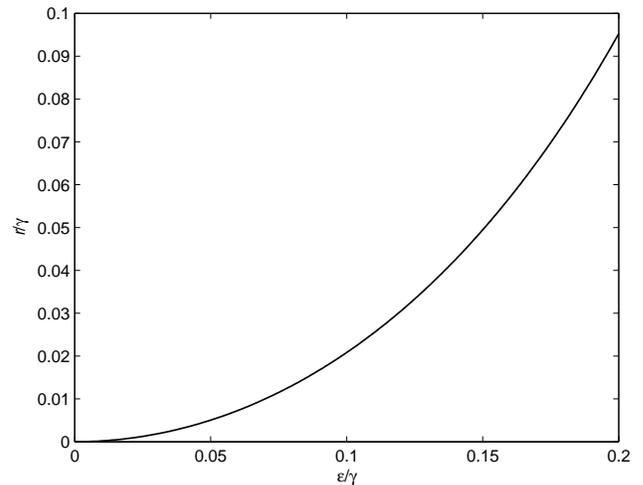
FIG. 5: Production rate  $r$  versus  $\epsilon/\gamma$  for  $\eta_t = 1$ .
