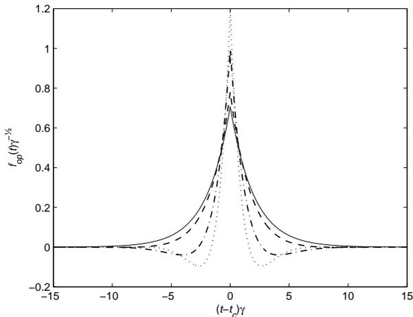
FIG. 3: Optimal mode function  $f_{op}(t)$  for  $\epsilon/\gamma = 0$  (solid line),  $\epsilon/\gamma = 0.1$  (dashed line),  $\epsilon/\gamma = 0.2$  (dot-dashed line), and  $\epsilon/\gamma = 0.3$  (dotted line). The signal detector efficiency is  $\eta_s = 1$ .
