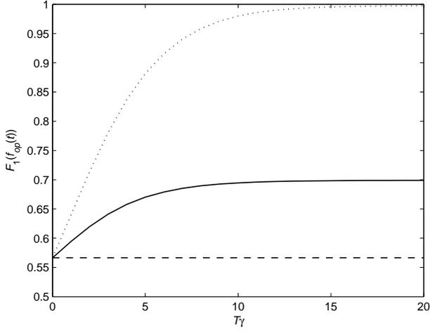
FIG. 6: Optimized one-photon fidelity as a function of vacuum detection window  $T$ . The trigger detector efficiency is  $\eta_t = 1$  for the dotted line,  $\eta_t = 0.4$  for the solid line, and  $\eta_t = 0$  for the dashed line, while  $\epsilon/\gamma = 0.2$  for all curves.
