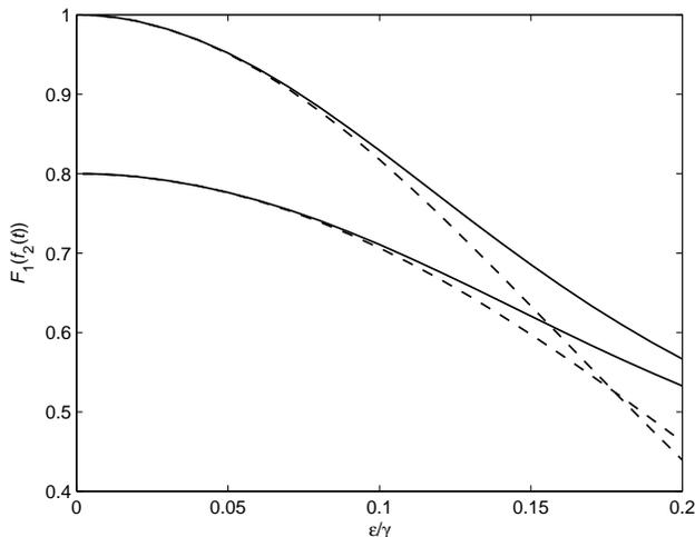
FIG. 4: Fidelity calculated from the numerically optimized mode function (solid lines) and from the  $\epsilon = 0$  mode function in equation (20) (dashed lines). The curves approaching 1 for small  $\epsilon$  are for perfect detection  $\eta_s = 1$ , and  $\eta_s = 0.8$  for the curves approaching 0.8 for small  $\epsilon$
