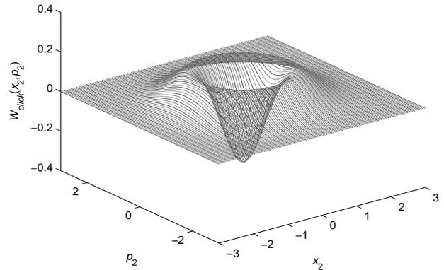
FIG. 2: Wigner function conditioned on a single trigger detector click event for  $\epsilon/\gamma = 0.02$ ,  $\eta_s = 1$ , and  $f_2(t) = \sqrt{\gamma/2} \exp(-\gamma|t - t_c|/2)$ . The one-photon state fidelity is 0.9921, and the negativity at the origin is  $W_{click}(0, 0) = -0.3133$ .
