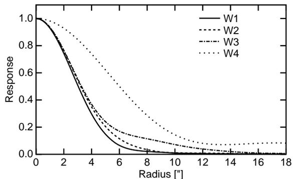
Fig. 11.— Azimuthally averaged point spread functions for WISE.
