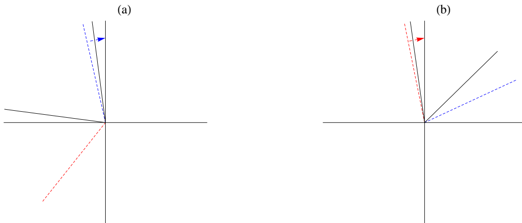
FIG. 5: Turning points entering and leaving the K = 1 wedge as \epsilon increases. As \epsilon increases past 1, the K = 1 turning point, whose angle is indicated by a dotted line, leaves the wedge, as shown by the arrow [panel (a)]. Then, as \epsilon increases past 3, a new turning point enters the wedge [panel (b)].
