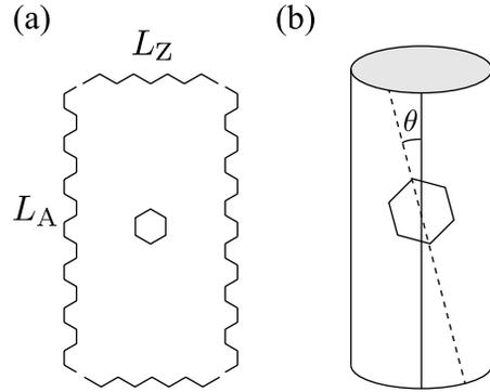
Fig. 1. (a) Chirality of a GNR. A large aspect ratio  $L_Z/L_A \gg 1$  ( $L_Z/L_A \gg 1$ ) defines an armchair (zigzag) GNR, where  $L_A$  and  $L_Z$  denote the lengths of the armchair and zigzag edge, respectively. (b) The chirality of a CNT is defined by the angle  $\theta$  with respect to the direction of the CNT axis.
