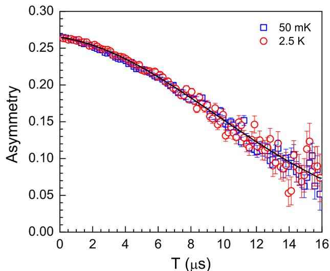
FIG. 8. (colour online) Zero field  $\mu$ SR spectra measured in longitudinal geometry below (50 mK, squares) and above (2.5 K, circles) the superconducting transition temperature. The solid line is the fit to the Gaussian Kubo-Toyabe function as described in the text.
