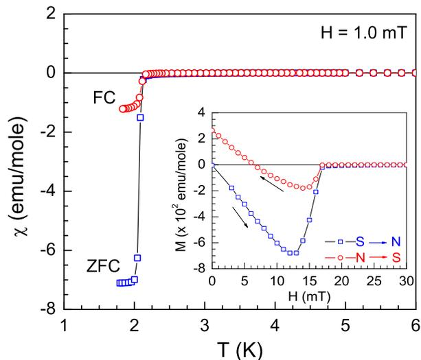
FIG. 2. (colour online) Temperature dependence of low temperature zero field cooled (ZFC) and field cooled (FC) magnetic susceptibility  $\chi(T)$  data of  $\text{LaRhSi}_3$  measured at 1.0 mT. The inset shows the isothermal magnetization as a function of magnetic field measured at 0.5 K. Arrows indicate the directions for the magnetic field cycle between the normal (N) and superconducting (S) states.
