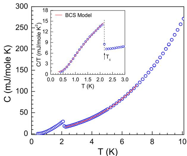
FIG. 4. (colour online) Specific heat  $C(T)$  data of  $\text{LaRhSi}_3$  as a function of temperature measured in zero field. The solid line (above  $T_c$ ) is a fit to  $C = \gamma T + \beta T^3$ . The inset shows the expanded view near the superconducting transition, plotted as  $C/T$  vs.  $T$ . The solid line in the inset represents the theoretical temperature-dependent spin-singlet fully gapped superconductor according to the weak coupling BCS model as tabulated by Mühlischlegel, Ref. 23.
