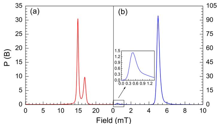
FIG. 10. (colour online) The maximum entropy spectra for (a) 15.0 mT at 0.2 K, and (b) 5.0 mT at 0.2 K. Inset in (b) shows an expanded view to show the increase in  $P(B)$  near  $B = 0$ .
