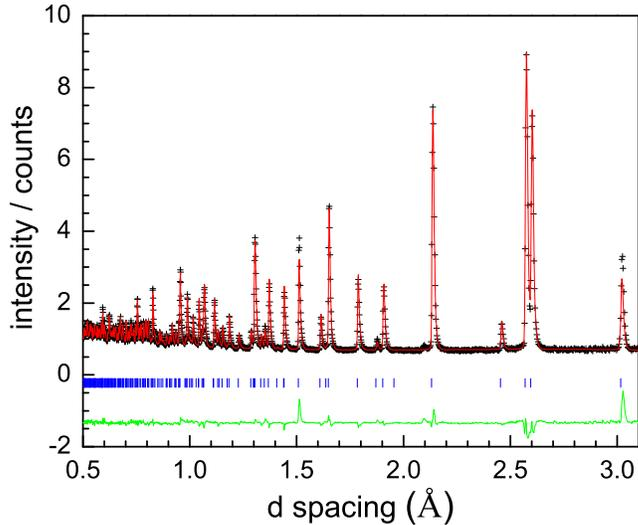
FIG. 1. (colour online) Neutron diffraction pattern of  $\text{LaRhSi}_3$  recorded at room temperature. The solid line through the experimental points is the Rietveld fit profile using the  $\text{BaNiSn}_3$ -type tetragonal structure (space group  $I4mm$ ). The short vertical bars mark the theoretical Bragg diffraction positions. The lowermost curve represents the difference between the experimental and calculated results.
