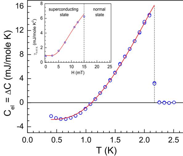
FIG. 5. (colour online) Temperature dependence of the electronic part of the specific heat,  $C_{el}(T)$  of  $\text{LaRhSi}_3$ , the solid line is the fit assuming an isotropic s-wave BCS superconducting gap,  $C_{el}(T) \sim T^{1/2} \exp(-\Delta_0/k_B T)$ . The inset shows the field dependence of  $\gamma$ , where the solid line represents an exponential evolution of  $\gamma$  under the application of magnetic field.
