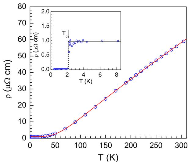
FIG. 3. (colour online) Electrical resistivity of LaRhSi<sub>3</sub> as a function of temperature measured in zero magnetic field. The solid line represents our fit to the Bloch-Grüneisen model. The inset shows the expanded view of the low temperature data showing the superconducting transition. The lines are drawn as a guide to the eye.
