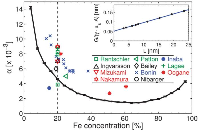
FIG. 5: Calculated zero temperature (solid line) and experimental room temperature (symbols) values of the Gilbert damping parameter as a function of the concentration  $x$  for fcc  $\text{Ni}_{1-x}\text{Fe}_x$  binary alloys<sup>17,18,120–131</sup>. Inset: total damping of  $\text{Cu}[\text{Ni}_{80}\text{Fe}_{20}]\text{Cu}$  as a function of the thickness of the alloy layer. Dots indicate the calculated values averaged over five configurations while the solid line is a linear fit.
