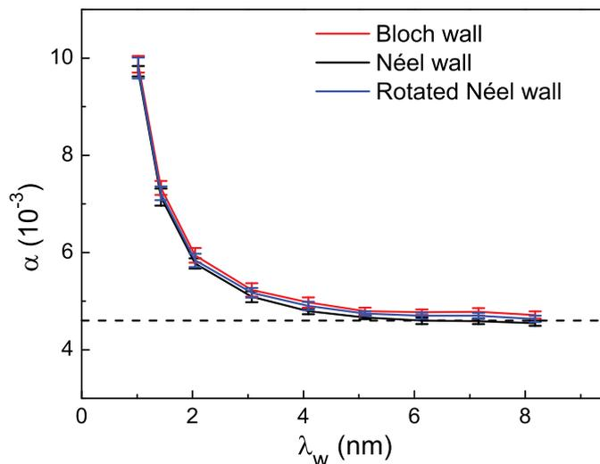
FIG. 8: Calculated effective Gilbert damping constant  $\alpha$  for Py DWs as a function of  $\lambda_w$ . The dashed lines show the calculated  $\alpha$  for bulk Py with the magnetization parallel to the transport direction<sup>89</sup>.
