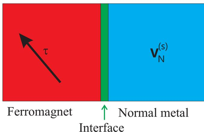
FIG. 1: Illustration of the spin-transfer torque in layered normal metal|ferromagnet system. A spin accumulation  $\mathbf{V}_N^{(s)}$  in the normal metal induces a spin-transfer torque  $\boldsymbol{\tau}_{\text{stt}}$  on the ferromagnet.
