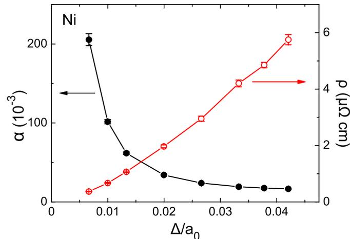
FIG. 6: Calculated Gilbert damping and resistivity for fcc Ni as function of the relative RMS displacement with respect to the corresponding lattice constant,  $a_0 = 3.524 \text{ \AA}$ .
