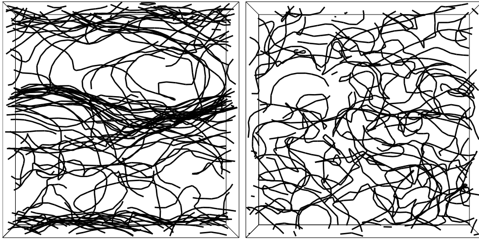
FIG. 11: Views of the tangles from the top of the computational domain in the xy -plane for the LIA simulation (left) and the tree method (right). The domain is a cube with sides of length 0.2 cm; the imposed normal velocity is v_{ns} = 0.5 cm/s and T = 1.6 K. Note the stratified nature of the tangle wrongly predicted by the LIA.
