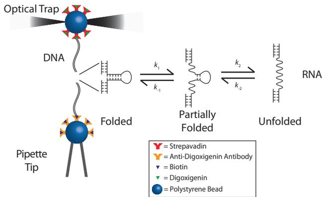
FIG. 1. **Single-molecule optical trapping configuration.** The biomolecule of interest—here, the p5ab RNA hairpin—is tethered to two polystyrene beads by dsDNA handles. The fluctuating force on one bead held in an optical trap is monitored, while the other bead is held suctioned to a micropipette tip. Conformational transitions of the hairpin—such as transitions among the three kinetically metastable states illustrated here—are observed indirectly through motion of the bead in the trap.
