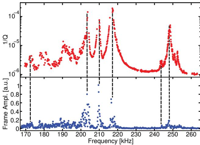
FIG. 3. Upper plot: spectrum of membrane dissipation  $Q^{-1}(f_{1,1})$ , showing a variation over two orders of magnitude. Lower plot: vibrations of the frame measured close to the membrane. The resonances in  $Q^{-1}(f_{1,1})$  coincide with the frame modes.
