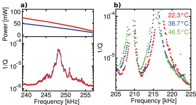
FIG. 4. a)  $f_{1,1}(P)$  and  $Q^{-1}(f_{1,1})$  for different heating laser positions (membrane center: blue, off-center: red). The spectra  $Q^{-1}(f_{1,1})$  overlap, indicating that  $Q$  is directly dependent on frequency. b)  $Q^{-1}(f_{1,1})$  for different sample holder temperatures. Heating shifts the frame modes to lower frequencies.
