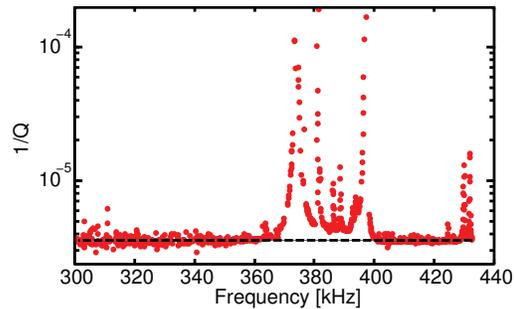
FIG. 5. Spectrum of membrane dissipation  $Q^{-1}(f_{1,1})$  for another membrane ( $l = 250$   $\mu\text{m}$ ,  $t = 50$  nm). Besides coupling to frame modes, the dissipation is independent of frequency.
