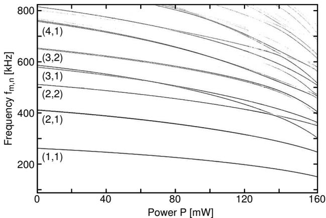
FIG. 2. Mode spectrum  $f_{m,n}$  of a membrane ( $l = 0.5$  mm, thickness  $t = 50$  nm) as a function of  $P$ . At  $P = 0$ , the lowest 13 modes lie within 2% of the expected frequency. At higher  $P$ , anticrossings between higher order modes are visible.
