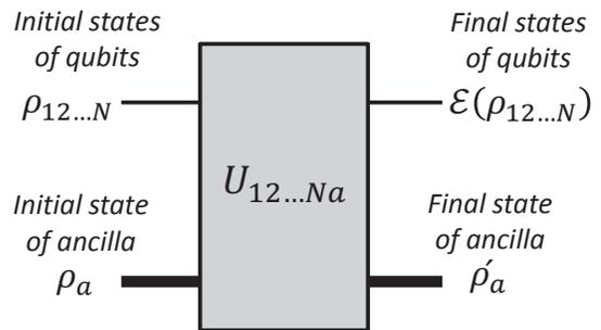
Figure 2. Ancilla-assisted implementation of entanglers viewed as a quantum operation  $\mathcal{E}(\rho_{12\dots N})$ . The joint ancilla-qubit system evolves under a unitary transformation  $U_{12\dots Na}$ .
