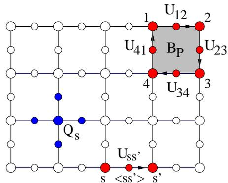
FIG. 1. In the lattice boson model, bosons live on both the sites  $s$  and links  $\langle ss' \rangle$  of the square lattice. The Hamiltonian  $H_B$  (1) is a sum of a  $Q_s$  term (2), which acts on four links  $\langle ss' \rangle$  and one site  $s$ , and a  $B_P$  term (4), which acts on the four sites and links adjacent to a plaquette  $P$ . The  $B_P$  term is a product of four link operators  $U_{ss'}$  (5) which each act on the sites  $s, s'$  and the link  $\langle ss' \rangle$ .
