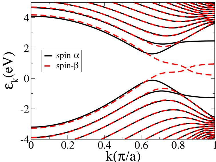
Figure 8: (Color online) Band structure of ZGNR-14 in the presence of external electric field ( $E_y = 2$  V/nm), obtained by P-P-P-UHF method. The solid-black (dotted-red) lines represent the bands of  $\alpha(\beta)$ -spin electrons.
