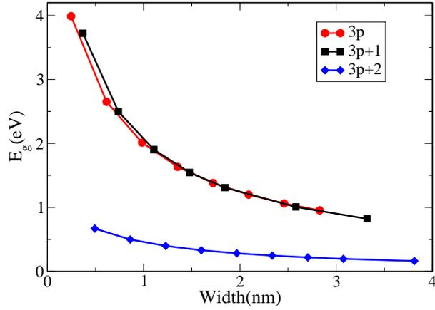
Figure 3: (Color online) Variation of the band gaps of AGNRs- $N_A$ , for  $N_A = 3p$ ,  $3p + 1$ , and  $3p + 2$ , families, with respect to their width. All calculations were performed with the original screened parameters ( $U = 8.0$  eV and  $\kappa_{i,j} = 2.0$  ( $i \neq j$ ) and  $\kappa_{i,i} = 1$ )(author?) [52] in the P-P-P model.
