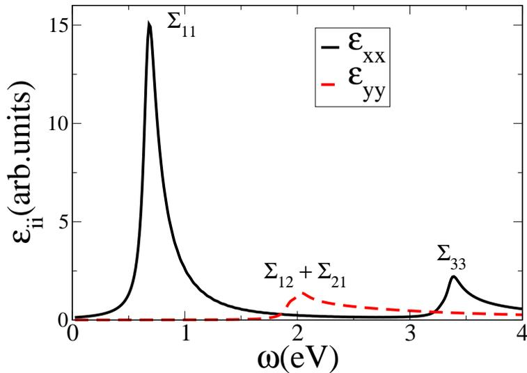
Figure 9: (Color online) Optical absorption spectrum of AGNR-14 obtained by P-P-P-RHF method. The solid-black line represents  $\epsilon_{xx}$ , while the dotted-red line represents  $\epsilon_{yy}$ . A line width of 0.05 eV was assumed.
