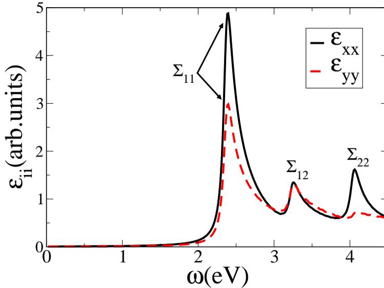
Figure 10: (Color online) Optical absorption spectrum of ZGNR-10 obtained by the P-P-P-UHF method. The solid-black line represents  $\epsilon_{xx}$ , while the dotted-red line represents  $\epsilon_{yy}$ . A line width of 0.05 eV was assumed.
