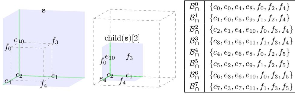
FIG. 4.1. (left) An illustration of a specific instance of Proposition 4.1. If the range  $[f, 1]$  contains only descendants of  $\text{child}(s)[2]$ , then its domain intersects  $\text{Dom}((s, b))$  (left) if and only if it intersects  $\text{Dom}((\text{child}(s)[i], b))$  (right) and  $b \in \mathcal{B}_\cap^2$ . (right) The child-boundary intersections are enumerated.
