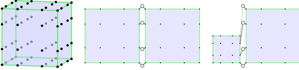
FIG. 6.1. (left)  $Q^n$ -nodes for  $n = 3$ , with one node at each corner,  $n - 1$  nodes on (the interior of) each edge,  $(n - 1)^2$  nodes on each face, and  $(n - 1)^3$  nodes in each element. (middle, right) For both conformal and non-conformal interfaces, each element node corresponds to exactly one global node. (right) At non-conformal interfaces, an element may reference a global node remotely, as the small element references the top node.
