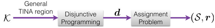
Fig. 3: The exact solution, where the disjunctive program identifies the optimal GDoF tuple \mathbf{d} in which the links in the subset \mathcal{S} with positive GDoF values are scheduled, and the assignment problem outputs the power allocation vector \mathbf{r} .
